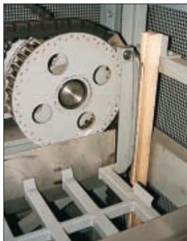
Driven wheel, plastic guide rail and platform from a circulating vertical conveyor for unit loads of varying dimensions.
